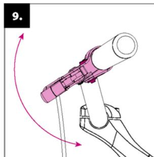
**Adjustment of brake levers:** incline the brake levers correctly by loosening the screw on the sleeve.
