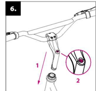
Insert the handlebar tube into the front frame (1) and adjust the height according to the rider's needs (not higher than indicated by the line). Check that the handlebar is upright and properly tighten the screw on the handlebar tube (2).
