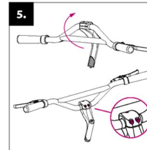
**Handlebar installation:** place the handlebar tube as shown on the picture and tighten the screws on the stem.
