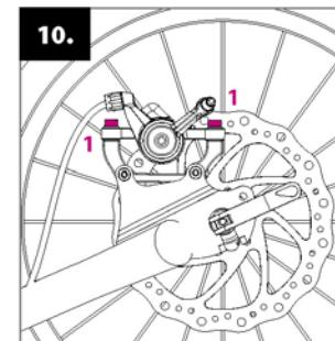
**Adjustment of brakes:** on both wheels, check that the discs are not touching the brake pads when the wheel is turning. If yes, loosen the adjusting screws (1) and regulate the position of both brake pads so that they are parallel to the disc on their whole length. Then tighten the screws again.
