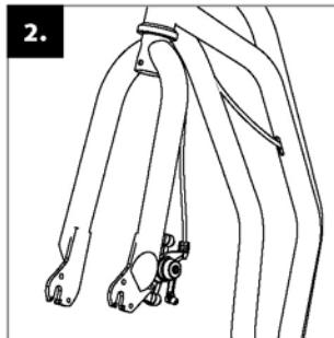
Make sure the front fork of the scooter is well positioned (disc brake is on the left side in rider's view).
