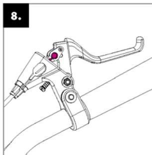
**Installation of brake cables:** press the brake lever to the maximum and insert the ending of the brake cable into the circular fixing point. Repeat the action with both brakes.
